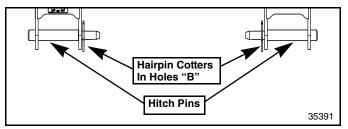
3-Point Hitch Pin Configuration For Cat. II Hitch And Quick Hitch Pin Configuration For Cat. I & II Hitches Figure 1-7
